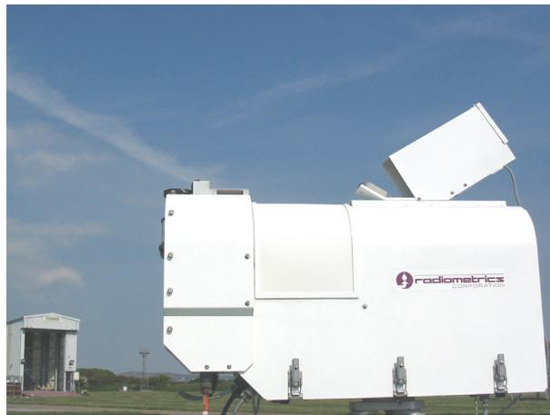
**Figure 1-4 Radiometrics TP/WVP-3000 Microwave Radiometer System at Camborne.**
