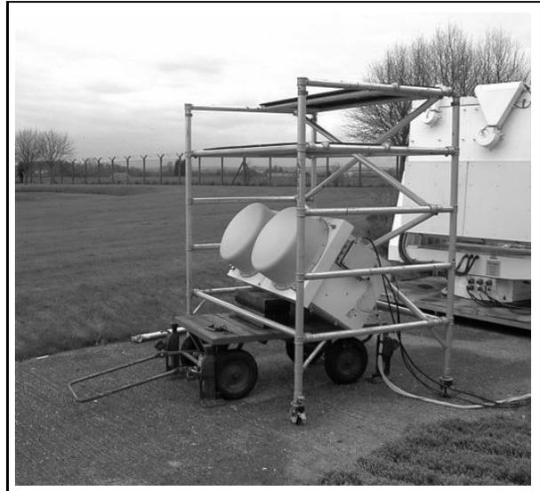
FIG. 6: Photograph of the *Galileo* radar on 14 March 2002. The elevation angle was  $30^\circ$  and the scaffold provided shelter from the rain. The radar was pointed to the west and the wind direction in the two days that it was inclined at this angle was weak easterly.
