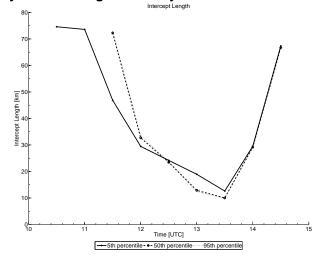
**Figure 3.** The Intercept Length, computed from the algorithm of Roberts and Lean (2008) using the radar-derived two hour accumulations at 5 km grid spacing as observations. Values larger than 80 km are not plotted. Note that the intercept lengths for the 50<sup>th</sup> and the 95<sup>th</sup> percentiles are almost identical.
