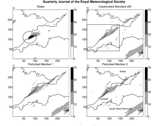
Figure 1. Rainfall accumulations in mm from 1200 to 1700 UTC 16 August 2004 for: a) radar observations (5 km grid length) with the target area circled (see Sec 4.1), b) the control simulation with the area used to compute the cloud profiles marked (as described in Sec 5.4), c) and d) two members of the model-state perturbed control ensemble. The star in c) marks the location of the town of Boscastle. The axis labels indicated the distance in km, from the South West corner.
