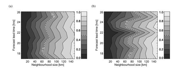
FIG. 6. FSS calculations over the Edinburgh subdomain: (a) dFSS mean and (b) eFSS mean. The  $99^{th}$  percentile threshold is considered. The white dashed line at 0.5 represents the believable scale.
