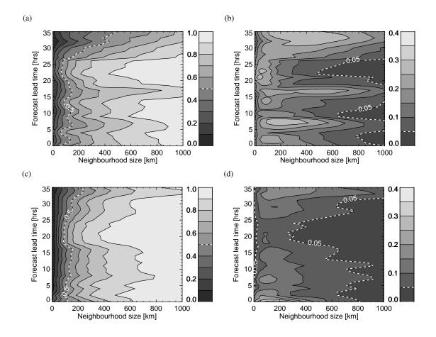
FIG. 7. dFSSmean (a,c) and dFSSstdev (b,d) for the organized Spring case (top) and the flooding case (bottom). The white dashed line in (a,c) at 0.5 represents the believable scale. To guide the eye, in (b,d) the white dashed line at 0.05 represents the neighborhood at which dFSSstdev is an order of magnitude smaller than the believable scale. The  $99^{th}$  percentile threshold is considered and results are calculated over the whole UK domain.
