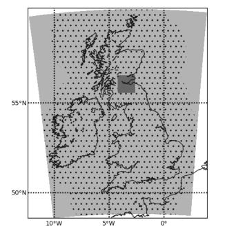
FIG. 2. Domains of the UK 2.2 km model (light gray), 100 km subdomain for the Summer flooding case (dark gray) and areas of radar coverage (dotted).
