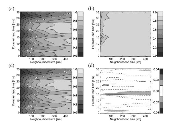
FIG. 10. dFSSmean comparisons of the restricted convection with increased time step and graupel physics configurations for the 99<sup>th</sup> percentile threshold of hourly precipitation accumulations. Results from different comparison strategies are shown: (a) MOGREPS2, (b)Physics2 and (c) MOGREPS2+Physics2. (d) shows the difference between sub-figures (c) and (a). Results are calculated over the whole of the UK domain. The white dashed line at 0.5 represents the believable scale.
