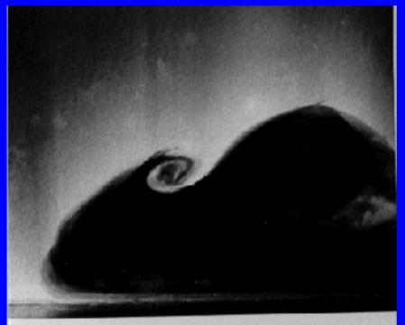
Figure 11.11 Laboratory photograph of less dense third mining above and below a gravity-current from Kelvin-Helmholtz billows form above: third ingested from below rises as it approaches the leading edge.
