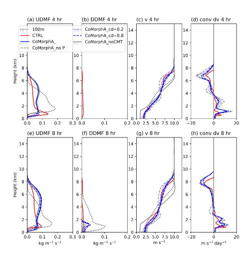
Fig 10. CMT. Profiles at 4 hours of (a) updraught mass flux [kg m<sup>-2</sup> s<sup>-1</sup>], (b) downdraught mass flux [kg m<sup>-2</sup> s<sup>-1</sup>], (c) meridional wind [m s<sup>-1</sup>] and (d) the increment in meridional wind due to convection [m s<sup>-1</sup> day<sup>-1</sup>] in the parameterized runs for the cold air outbreak case. (e-h) as (a-d) but 8 hours into the run. Results shown for the 100 m CRM (black), CTRL (red)
