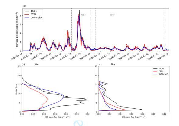
Fig 7. TWP-ICE. (a) Timeseries of 15-minute precipitation rates [mm hr<sup>-1</sup>] and mean updraught
