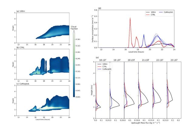
Fig 3.ARM. Time evolution of cloud fraction in (a) 100 m CRM, (b) CTRL and (c) CoMorph-A simulations of the shallow ARM case. (d) Timeseries of precipitation [mm hr<sup>-1</sup>] from the three simulations. (e) Updraught mass flux [kg m<sup>-2</sup> s<sup>-1</sup>] profiles between 1800 and 2300 local time. (d) and (e) are shown for each ensemble member (thin lines) and the ensemble mean (thick line).
