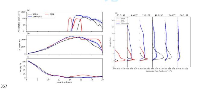
Fig 4.AMMA. Timeseries of (a) surface precipitation [mm day-1], (b) boundary layer depth [m] and (c) CIN [J Kg-1] from the 100m CRM (black), CTRL (red) and CoMorph-A (blue) ensemble members (thin lines) and ensemble mean (thick line) simulations of the AMMA case. (d) Hourly mass flux [kg m<sup>-2</sup> s<sup>-1</sup>] profiles from 1300 to 1800 local time.
