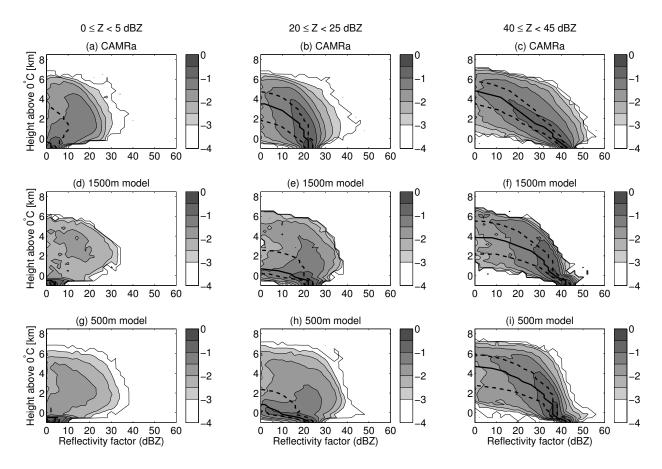
FIG. 7. As in Figure 6, but for the case of 25 August 2012. Rows are now in order: observations (first), UM at 1500-m grid length (second), UM at 500-m grid length (third). The 500-m simulation was run with 140 vertical levels.
