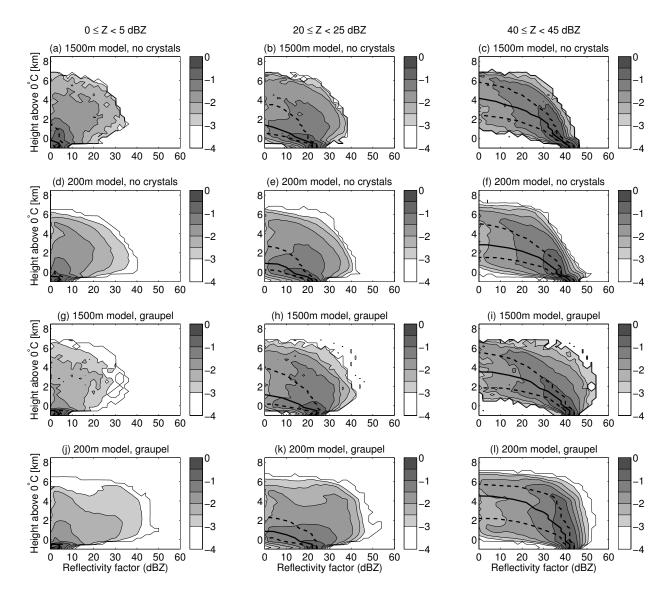
FIG. 9. As in Figure 7, but for the UM with all diagnostic ice set to be aggregates at 1500-m grid length (first row) and 200-m grid length (second); and the UM with graupel at 1500-m grid length (third) and 200-m grid length (fourth). Both 200-m simulations were run with 140 vertical levels.
