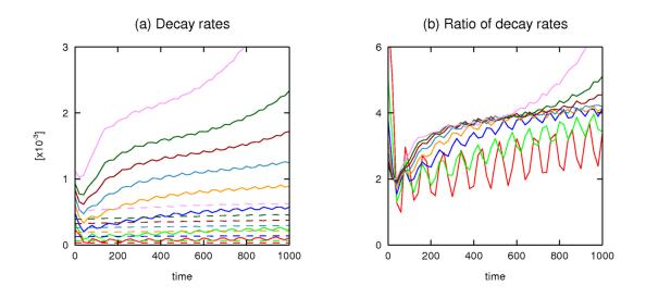
Figure 10: (a) Timeseries of the decay rate of primary wave amplitude for the full suite of diffusion experiments with  $\kappa = (0.25, 0.5, 1.0, 1.5, 2.0, 2.5, 3.0, 4.0) \times 10^{-6}$  (solid, with decay rates increasing with  $\kappa$ ) and the corresponding simulations with advection switched off (dashed). (b) The decay rates of primary wave amplitude in the full experiments divided by the same quantity in the corresponding simulations with advection switched off.
