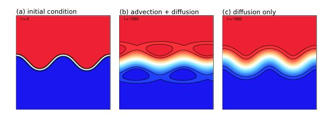
Figure 8: The PV field for an example simulation with diffusion parameter  $\kappa = 2 \times 10^{-6}$  at times (a) t = 0, and (b) t = 1000. Panel (c) shows the time t = 1000 state for the corresponding simulation with advection switched off (see text). In each panel the two outermost contours are marked by solid lines for clarity.
