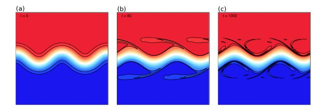
Figure 1: The PV field at times (a) t = 0, (b) t = 80, and (c) t = 1000 from the illustrative simulation with wave amplitude  $a = L_R$ , wavenumber  $k = 1/L_R$ , and smoothing width  $\sigma = 0.7L_R$ . In each panel the two outermost contours are marked by solid lines for clarity. The full  $1 \times 1$  model domain is shown. A movie of this simulation is provided in the supplementary material.
