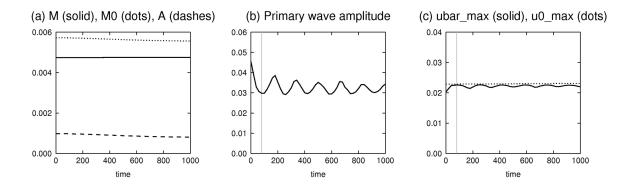
Figure 2: Timeseries of diagnostics from the simulation shown Figure 1: (a) M (solid),  $M_0$  (dots) and  $\mathcal{A}$  (dashed), (b) the primary wave amplitude, defined as the root mean square displacement of the q = 0 contour, and (c) the maximum magnitudes of the zonal mean zonal wind  $\bar{u}$  (solid) and reference state zonal wind  $u_0$  (dots). The vertical lines in panels (b) and (c) indicate the time t = 80.
