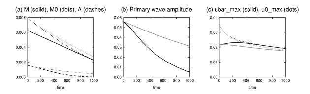
Figure 9: Timeseries of the same diagnostics as Figure 2 but for an example simulation with diffusion parameter  $\kappa = 4 \times 10^{-6}$  (black lines). The grey lines show the corresponding simulation with advection switched off.
